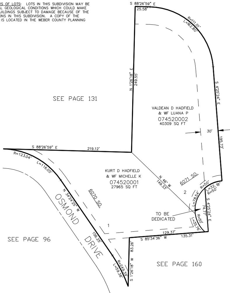
10' UTILITY & DRAINAGE EASEMENTS EACH SIDE OF PROPERTY LINES AS INDICATED BY DASHED LINES EXCEPT AS OTHERWISE SHOWN.
